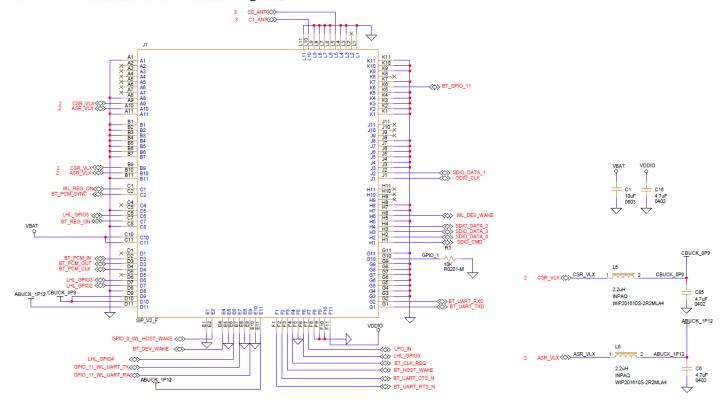
BT\_REG\_ON must be connected to an external GPIO control pin.
